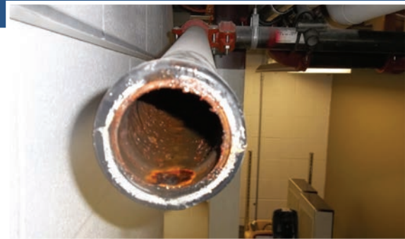
Corroded pipes may not activate a fire suppression system when needed, or activate it unexpectedly.
