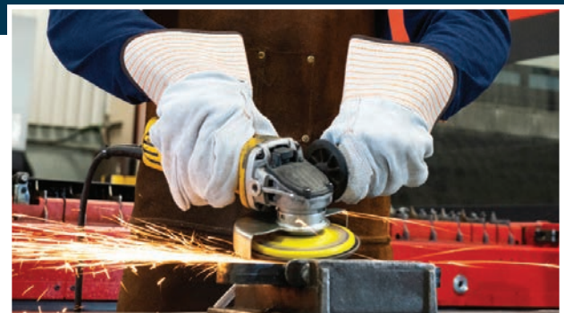
Vibration reducing gloves can help mitigate the effects of prolonged exposure to vibration.
