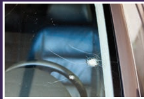
A cracked windshield from lawn mower debris is considered third-party damage and should be documented.
