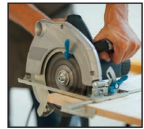
Saws should have guarding around the blade to help prevent accidental contact with the moving blade.
