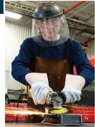
Wearing personal protective equipment is key to safe operation of abrasive wheel grinders.
