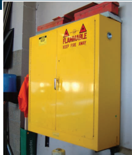
Flammable materials storage cabinet
